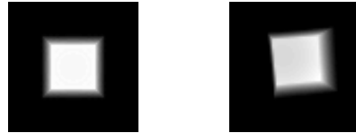
Fig. 4. The 2D projected images with (left) no rotation and translation and (right) rotations of (5^\circ, 5^\circ, 5^\circ) along each axis and translations of (0.1, 0.1, 0.1) pixels in the x -, y -, and z - directions.
