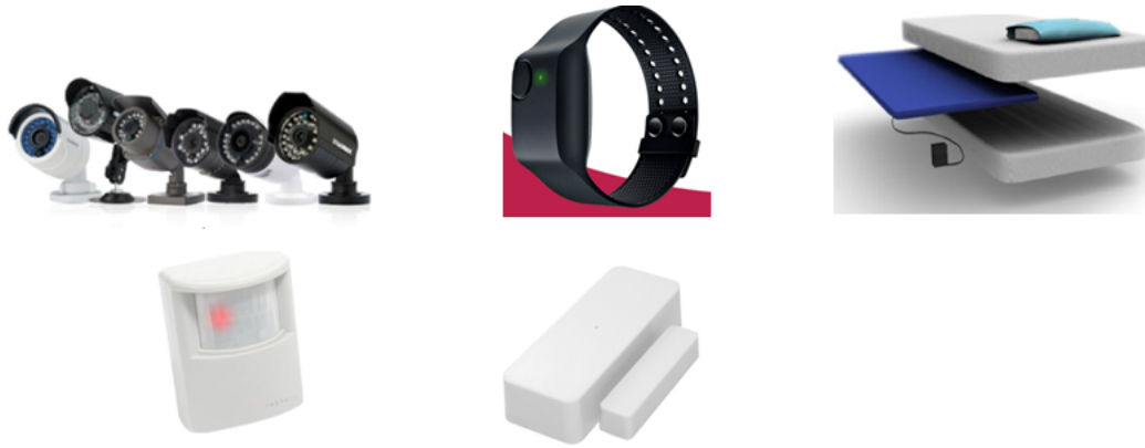
Fig. 1. Multimodal Sensors used in the study following the DAAD framework: (From Top Left in clockwise manner) Video Cameras, Empatica E4 wearable device, Pressure Mat, Motion Sensor, Door Sensor.
