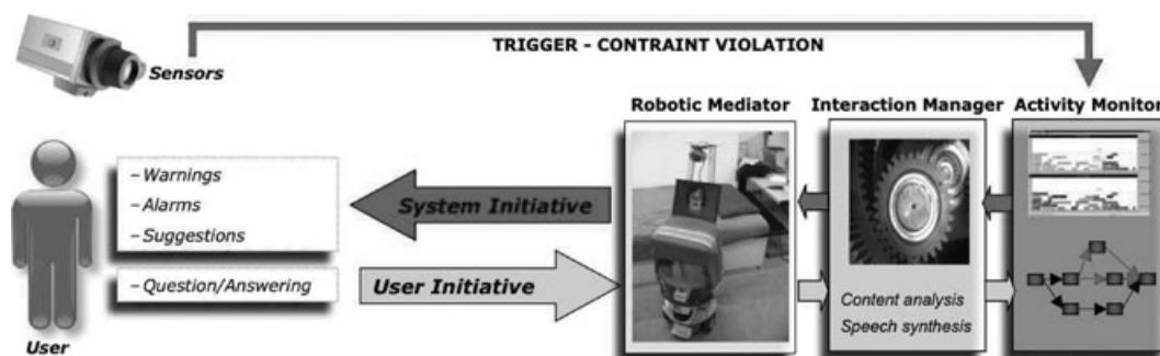
FIGURE 2. The general schema for mixed-initiative interaction generation in ROBOCARE.
