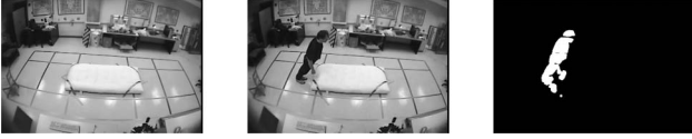
Fig. 3. Result of the moving object segmentation process. From left to right, background median model b_j , current frame i_j , and segmented picture s_j for camera j .
