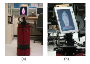
Figure 1: (a) HOMER the messenger robot (b) closeup of HOMER's head
