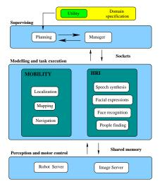
Figure 2: Control Architecture
