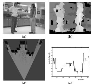
(d) (c) Figure 3: From stereo images to radial maps. (a) greyscale image (b) disparity image (black indicates invalid, otherwise brighter indicates closer to the cameras) (c) depth vs columns graph (depth in cm) (d) the resultant estimate of clear, unknown and occupied regions (light grey is clear, black is occupied and dark grey is unknown)
