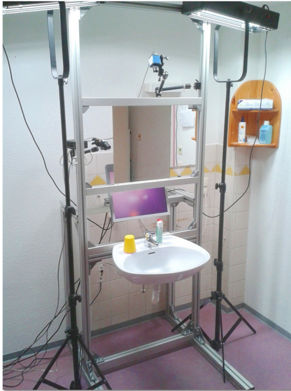
Fig. 2. Washstand setup equipped with sensor technology.
