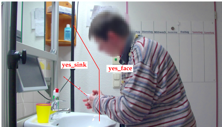
Fig. 9. Distinction between yes_sink and yes_face for variable brush_movement . In this example, the orientation of the brush (dashed line) points into the sink region and brush_movement is set to yes_sink .
