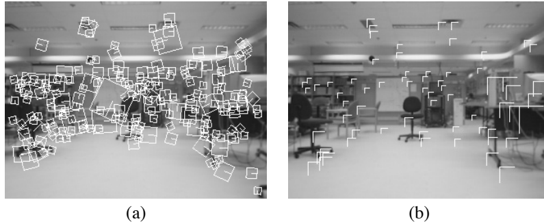
Figure 4: (a) SIFT features found, with scale and orientation indicated by the size and orientation of the squares. (b) Stereo matching result, where horizontal and vertical lines indicate the horizontal and vertical disparities respectively.
