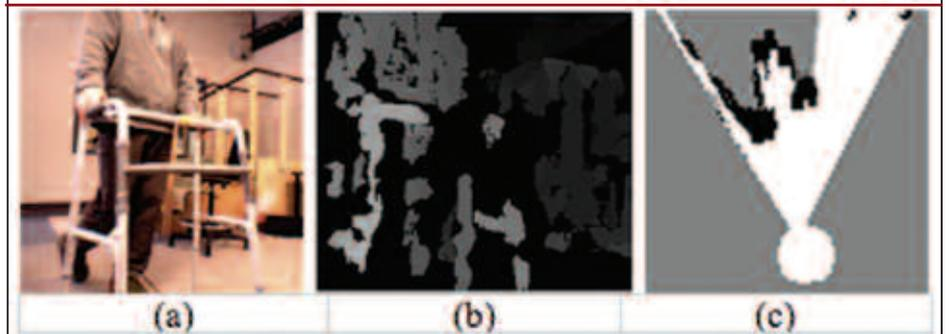
Images of a person standing in front of the wheelchair with a walker. Navigation maps are generated representing (a) camera view, (b) distance (depth) map and (c) 2D bird's-eye view of obstacles in the environment. In (b), the closer an object is, the brighter it appears. In (c), black represents known obstacles, white represents free space, and grey represents unknown regions.
