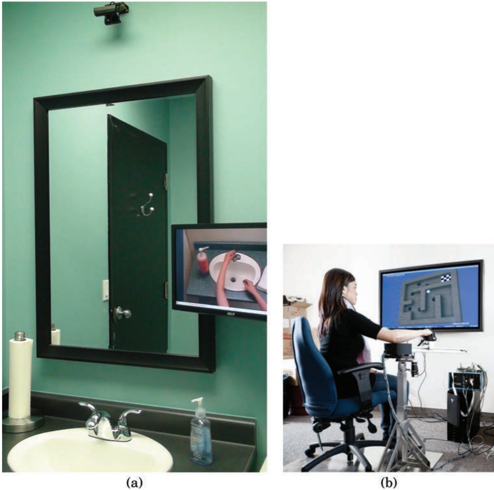
Fig. 4. (a) COACH handwashing assistant; (b) iSTRETCH haptic robotic device for stroke rehabilitation.
