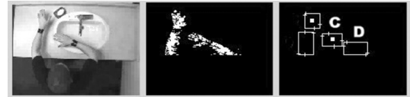
Fig. 3. Determining the right hand's location given two horizontally stacked blobs. The three frames illustrate the same stages of processing described in Fig. 2.
