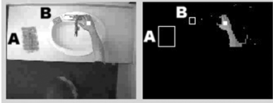
Fig. 5. Tracking both step-specific object and hand positions. The first frame shows the actual image from the frame, while the second frame illustrates the objects and hand being tracked after the HSI model (for the objects), NCC model (for the hand), and blob analysis (both types of objects) have been applied.
