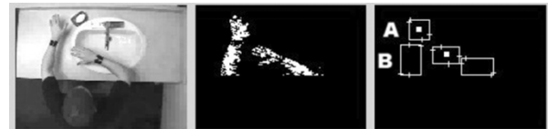
Fig. 2. Determining the hand's location given two vertically stacked blobs. The first frame represents the actual image from the video sequence, the second is the binarized image after the NCC model has been applied, and the third is a representation of the palm centers after blob analysis has been performed.
