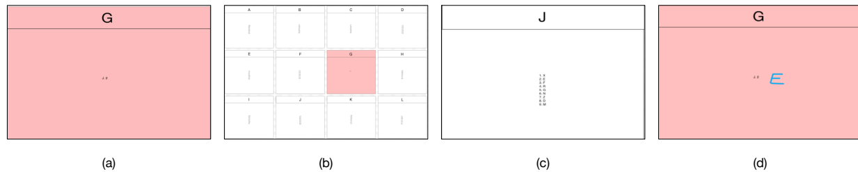
Figure 4. Navigation task. The user is presented with a detailed view of the starting cell, which shows the target cell and row (a). The user needs to zoom-out to locate the target cell (b), zoom-in to read the value (c) and finally return to the starting cell to write down the result (d).
