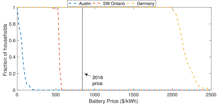
Figure 9. Fraction of households with non-zero optimal battery size as a function of the battery price.
