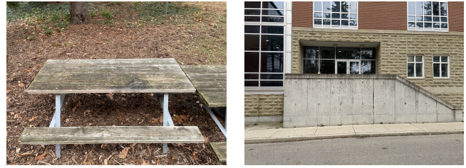
(a) Table with luminance of 2200 \text{ cd/m}^2 in direct sunlight. (b) Concrete with luminance of 5600 \text{ cd/m}^2 in direct sunlight.
