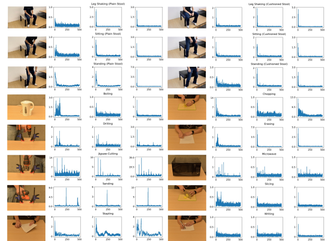
Figure 10: The tested activities and their frequency signatures on the X, Y, and Z directions of the accelerometer. In the signal plots, the X-axis represents frequency and the Y-axis represents magnitude.
