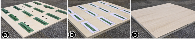
Figure 3: Fabrication process of an AccelLumber panel. (a) RF antennas are affixed to the bottom plywood layer using adhesive and mortise-and-tenon joints, with designated grooves for the PCBs. Note that the spacing between the antennas was determined based on the experimental results presented in the Appendix B. (b) Patch antennas are then placed into cutouts in the top layer, reinforced with polystyrene boards. (c) A wood grain contact paper is applied to the surface to provide the appearance of a wooden tile.
