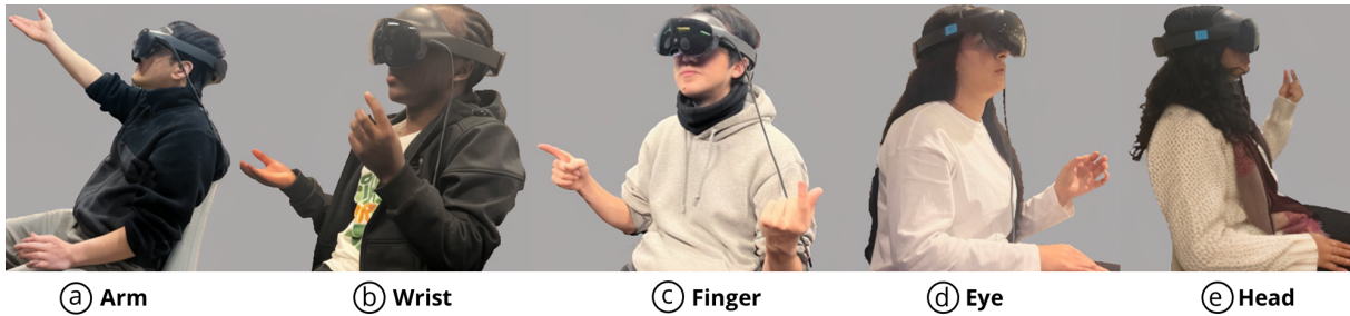
Figure 1: The five controller-free pointing techniques for study: (a) Arm, (b) Wrist, (c) Finger, (d) Eye, and (e) Head. Each was tested at 2, 6, and 10 meters of depth to evaluate movement time, error rate, throughput, and workload in AR 2D selection.
