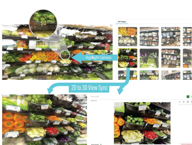
Figure 3: Hovering over a 2D image highlights its corresponding camera frustum in the 3D reconstruction. Clicking a 2D image automatically orients the 3D viewer to the associated camera pose and loads the selected image into the focused 2D viewer.
