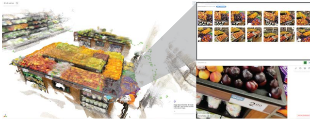
Figure 10: Label Information Retrieval. Users can select an item based on its spatial context and geometry in the 3D view, retrieve all images capturing that region, and examine the clearest image of the label or price tag in the 2D viewer.
