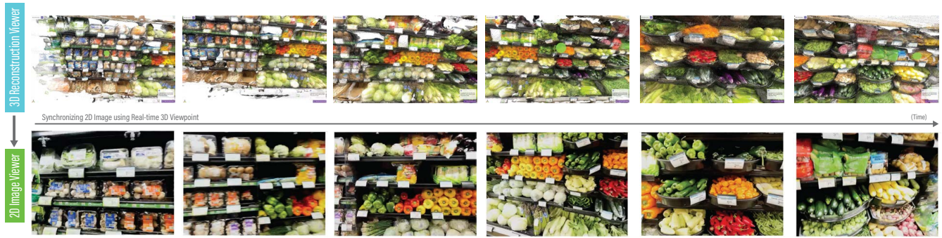
Figure 5: As the user navigates in the 3D Reconstruction Viewer (top), the system continuously updates and displays the closest 2D image (bottom) based on the current 3D viewpoint.
