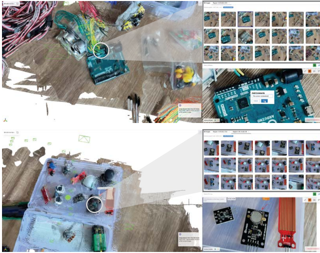
Figure 9: Hardware Review Scenario. Users inspect components in 3D, retrieve relevant 2D images to view wiring details, and leave persistent annotations for documentation.
