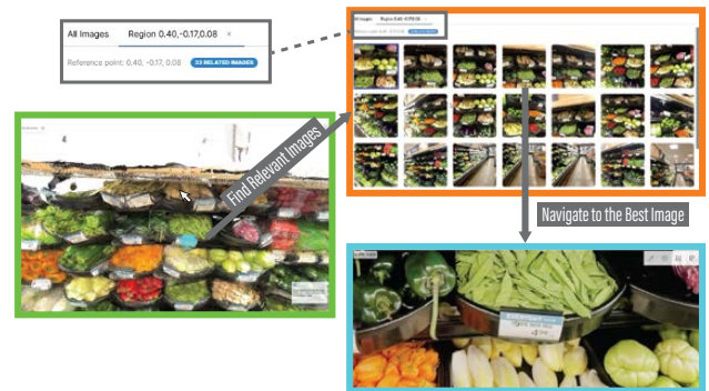
Figure 7: Clicking on a point in the 3D reconstruction triggers a spatial query that identifies nearby 3D points and retrieves all 2D images that capture that region. These relevant images are displayed in a new tab within the 2D image list, allowing users to select the optimal image for detailed visual inspection.
