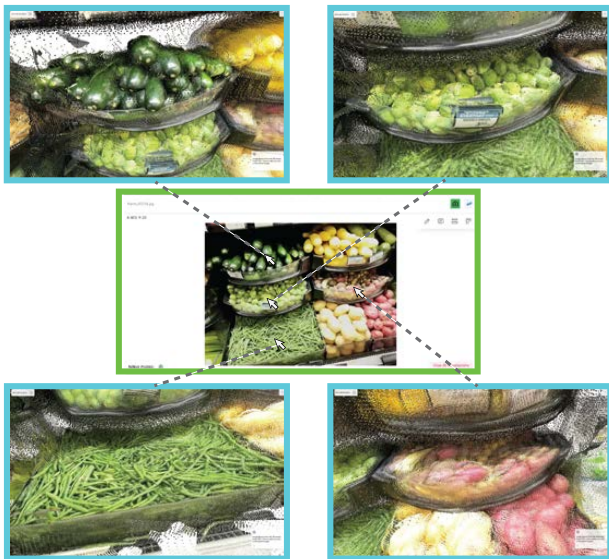
Figure 6: Users can click on a specific region within a 2D image, and the 3D viewer will automatically navigate to the corresponding location in the reconstruction.
