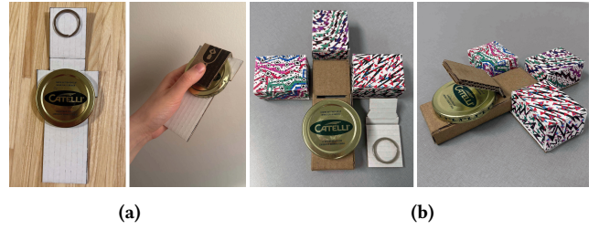
Figure 1: (a) Button prototype made of cardboard, metal lid, and key ring; user presses down to elicit a click. (b) Cardboard controller with button apparatus.
