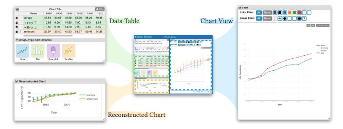
Figure 3: ChartDetective is composed of three views: the Chart View showing the chart being extracted; the Data Table with the tables for X and Y axes and the extracted values; the interactive Reconstructed Chart.
