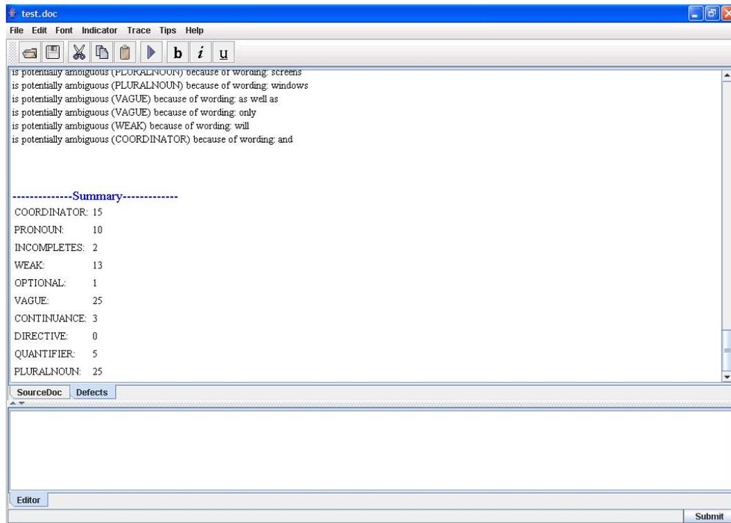
Figure 28. In the Defects tabbed pane, the Lexical Analyser reports a RStat with a description of the type of potential ambiguity
