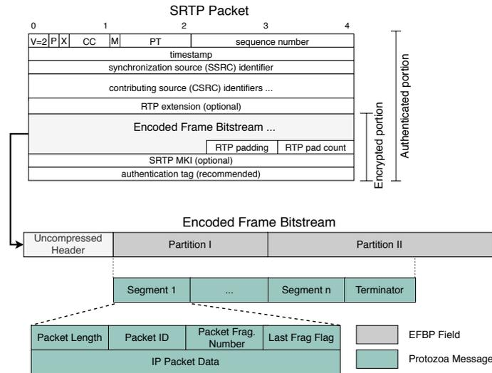
Figure 4.6: Format of SRTP packets: Protozoa replaces the EFBP payload containing carrier video bits with covert data.
