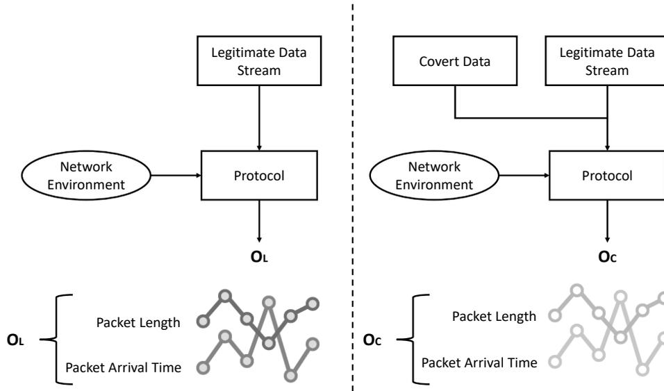
Figure 1.2: Overview of the protocol tunneling approach for the creation of covert channels.
