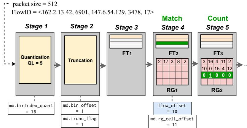
Figure 3.5: FMA implementation on Tofino switch. Each partition of the flow table ( $FT_m$ ) records flow ids (marked in orange) and their corresponding flow markers are recorded in the register grid partition of the upcoming stage ( $RG_m$ ). This packet is matched in  $FT_2$  and the respective flow marker updated in  $RG_2$ . The white boxes in the bottom indicate the metadata values computed in each stage; the value in the blue box is loaded by the control plane.
