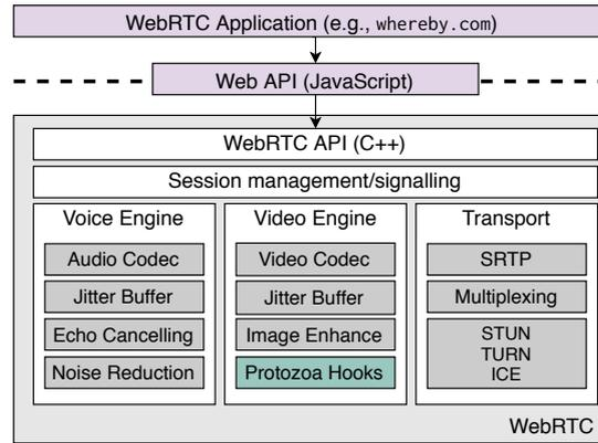
Figure 4.5: WebRTC software stack and Protozoa’s hooks.
