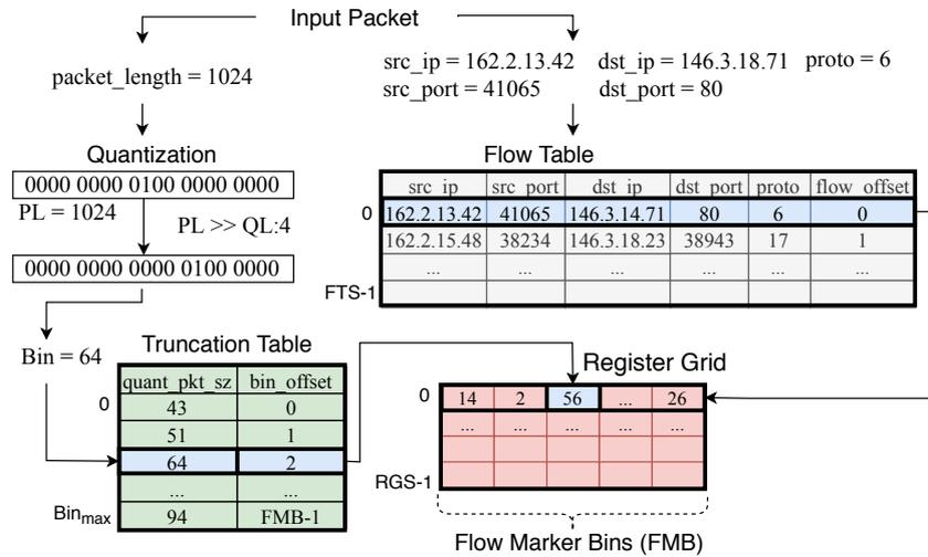
Figure 3.4: FMA internals: Flow Table, Truncation Table, and Register Grid.
