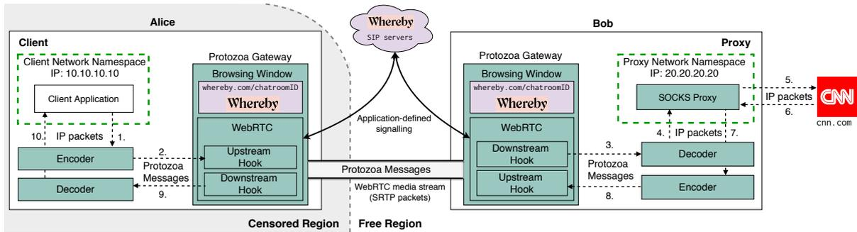
Figure 4.3: Architecture of Protozoa: The components of our system are highlighted.
