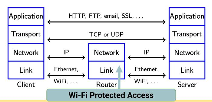
Cryptographic protection at the wireless data link layer
