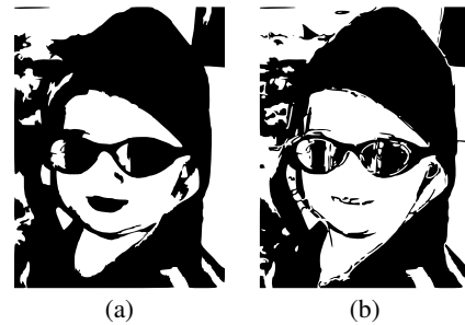
Figure 8: Demonstrations of the postprocessing operations discussed in Section 5. We smooth out isolated pockets of black and white in (a) using graph-based morphological operators. In (b), we superimpose edges between high-contrast segments that were assigned the same binary value.
