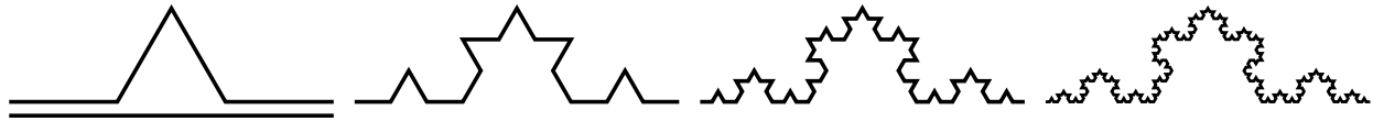
Figure 1 : The construction of the Koch curve. On the left, a unit line segment is shown with the base curve above it. The other three drawings show the evolving curve after one, two and three rounds of substitution.
