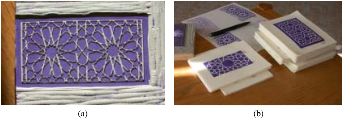
Figure 3.36 Examples of star patterns created using a CNC milling machine. The milling machine was used to route star patterns into linoleum printing blocks, from which hand prints were made.
