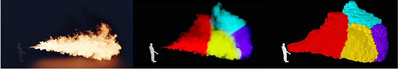
Fig. 9. Flamethrower. A volumetric combustion simulation (left) was run on 4 machines with our Power partitioner. Here fire/smoke density (middle) and sparse simulation domain buckets (right) are colored by rank. © Wētā FX Ltd.
