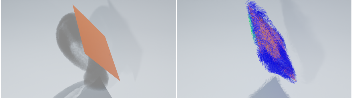
(b) Plane — A simple simulation of an open surface. Although the bottom side's flow moves quite quickly the flow is nearly static on the top.
