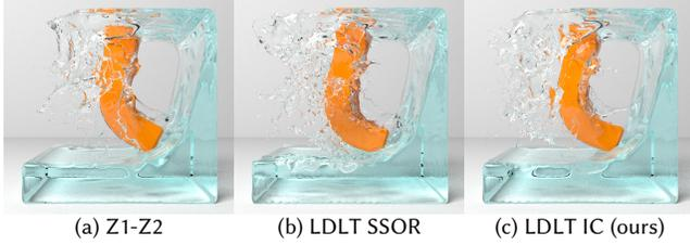
Fig. 7. An elastic beam (with its top fixed) deformed in a dam break scenario, simulated with different schemes (see §4.2). These approaches generate comparable visual results, but ours is at least  $4.7\times$  and  $2.9\times$  faster than Z1-Z2 and LDLT SSOR, respectively.
