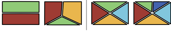
Figure 3: Regular and irregular vertex configurations in 2D: Left: An interface separating two regions is regular, as is a triple-point vertex separating three regions. Right: Vertices with edge valence of four or higher are irregular.
