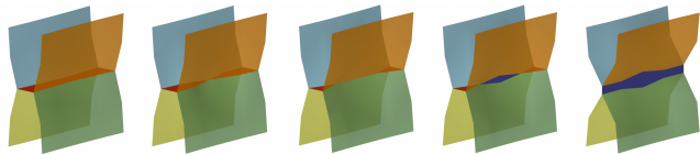
Figure 5: A 3D T1 process begins when a short edge between distinct triple-junction curves collapses to become a vertex incident on four materials. Adjacent edges on the original interface (red) also collapse yielding a quadruple-junction curve. Then, one vertex on the curve separates perpendicularly to create a new interface (dark blue). Nearby vertices follow suit to complete the process.
