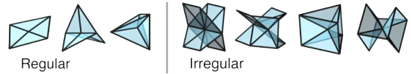
Figure 6: Regular and irregular configurations in 3D: Left: (1) A manifold surface separating two regions (here, the top and bottom half-spaces), (2) a triple-curve bordering three regions, and (3) a quadruple-point at which four regions meet. Right: Four of the infinitely many possible irregular non-manifold configurations that must be resolved by vertex separation.
