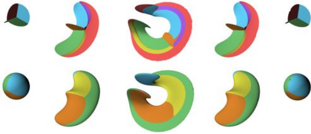
Figure 14: Multimaterial Enright test: A sphere divided into four material regions is advected through the “Enright test” velocity field. The distinct regions are well-preserved despite the extreme stretching. Top: Interior interfaces. Bottom: Exterior interfaces.
