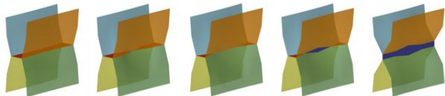
Figure 5: A 3D T1 process begins when a short edge between distinct triple-junction curves collapses to become a vertex incident on four materials. Adjacent edges on the original interface (red) also collapse yielding a quadruple-junction curve. Then, one vertex on the curve separates perpendicularly to create a new interface (dark blue). Nearby vertices follow suit to complete the process.
