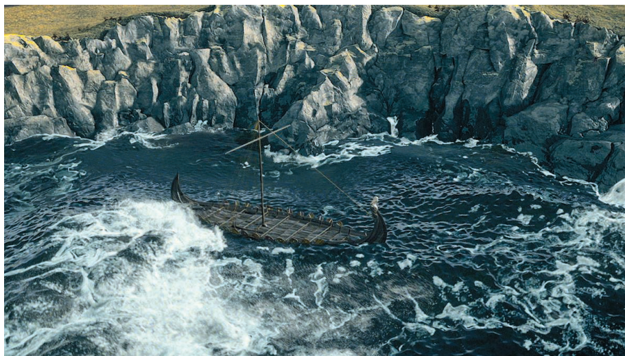
Realistic simulations. A simulated ship upon a simulated ocean. Here, the film industry's Naiad software is used to evolve the incompressible Navier-Stokes equations for the water, strongly coupled with the rigid-body dynamics of the longboat, with additional phenomenological simulation of foam and spray.
