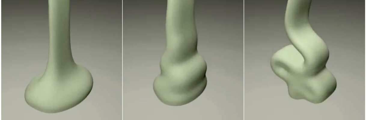
Figure 3: Three different simulations of a long sheet of fluid falling under gravity demonstrating the influence of viscosity on buckling; from left to right viscosity values are 0.2, 1, and 5.
