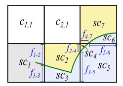
**Figure 5:** Geometry and notation used in our 2-D Poisson matrix example (Table 1). The solid thin boundary is shown in green.  $c_{i,j}$  is a regular grid cell at row j, column i.  $sc_k$  is sub-cell k.  $f_{a-b}$  is the fraction of the fluid edge shared by sub-cells a and b.
