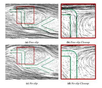
**Figure 10:** Flow simulation on a turning and branching tube whose width is smaller than a grid cell width. (a) Free-slip flows smoothly. (c) No-slip halts in the tube. (b) and (d) show closeup views of the highlighted regions.
