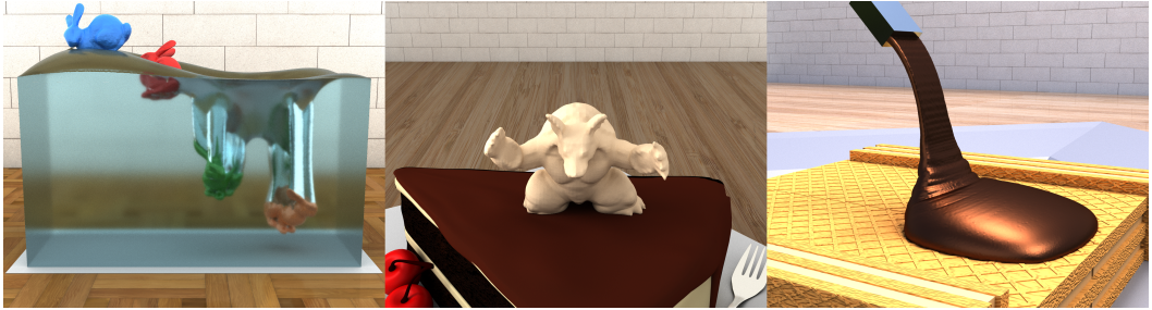
Fig. 1. (Left) Four bunnies of different masses are two-way coupled to a viscous liquid ( 384^2 \times 192 grid). (Middle) A creamy armadillo cake topping collapses under gravity ( 512^3 grid). (Right) Chocolate buckles as it pours onto a wafer ( 256^2 \times 512 grid).
