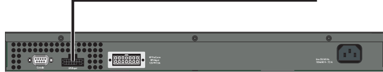
Figure 3-1. Example of an HP 600 RPS/EPS Powering One 2626-PWR Switch
