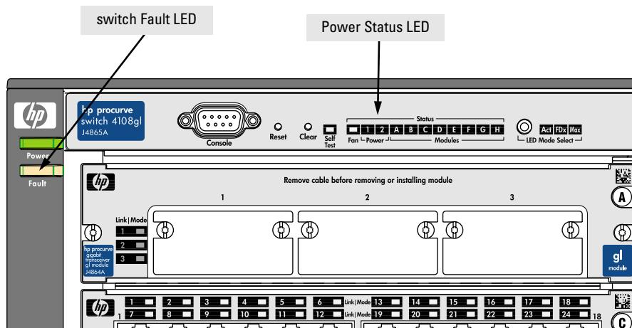
The Power Status LED for the power supply you have just installed will be blinking simultaneously with the Fault LED until that new power supply is connected to an AC power source. Once it is connected to AC power, the Power Status LED will be on continuously and not blinking, and the Fault LED will stop blinking.
