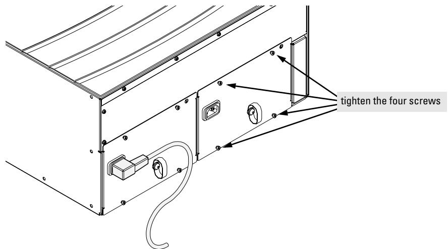
4. **Connect the power cord** supplied with the power supply to the power connector, and then into a properly grounded electrical outlet. To provide true redundancy, the second power supply should be connected to a different AC power source from the other supply. Then, if one AC power source fails, the switch will continue to run.
