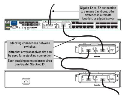
3. When the transceiver is receiving power and the stacking cable is connected to another active switch, the Link LED for the transceiver port should be ON.
