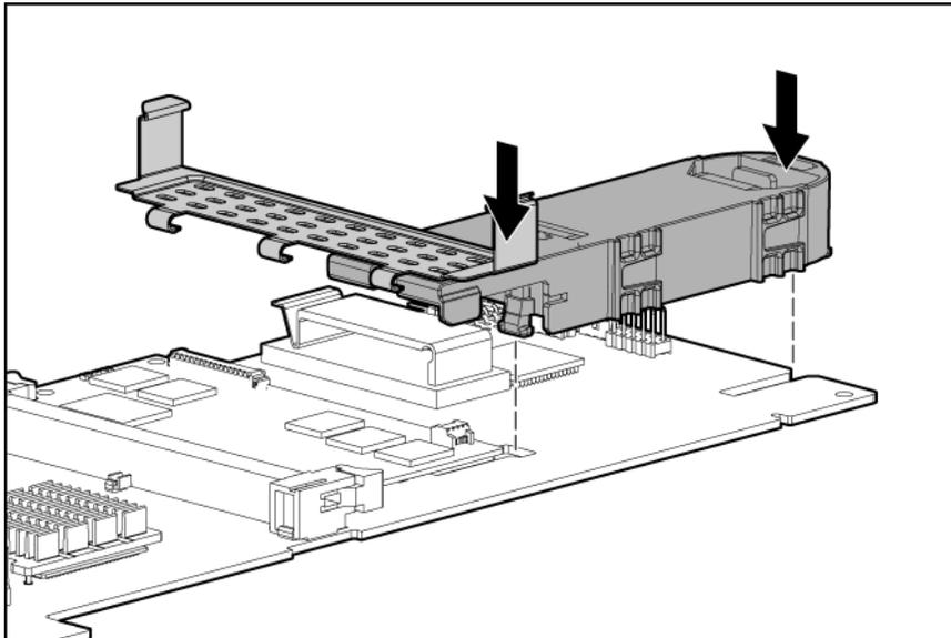
**CAUTION:** When connecting or disconnecting the capacitor pack cable, the connectors on the cache module and cable are susceptible to damage. Avoid excessive force and use caution to avoid damage to these connectors.
