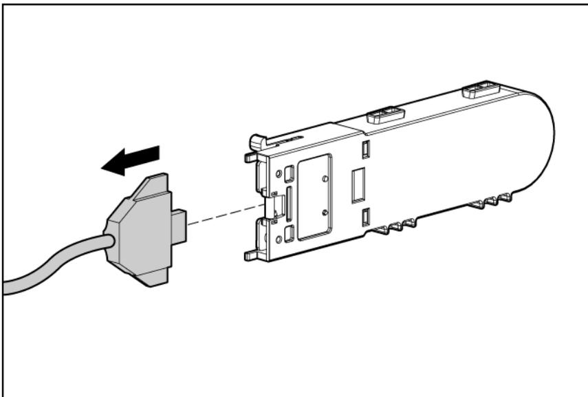
7. Connect the battery cable to the new battery.
