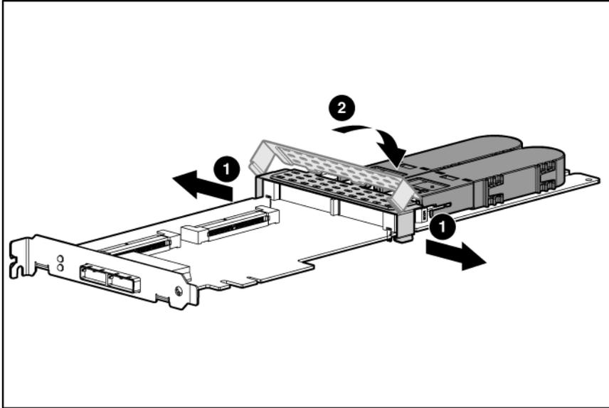
5. Slide the batteries toward the right edge of the controller, away from the bracket.
