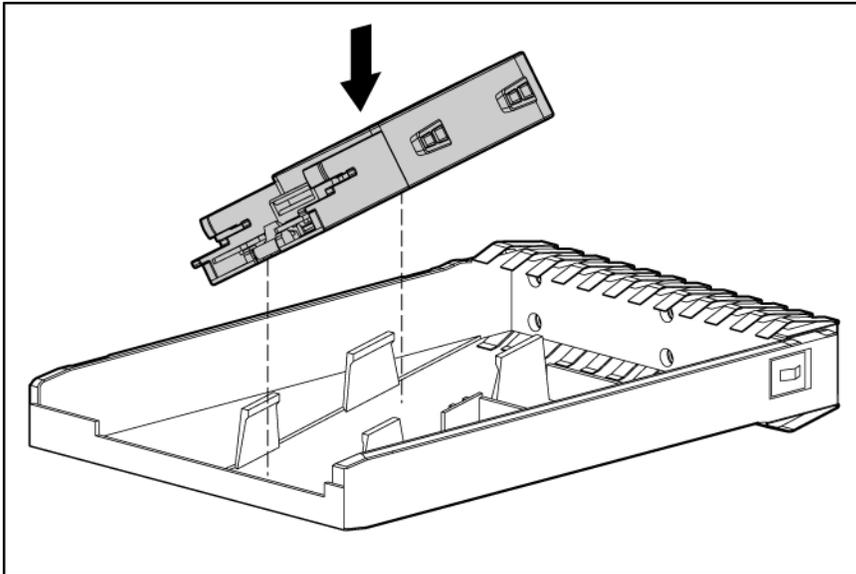
11. Pull the right-hand portion of the battery case away from the battery pack, and simultaneously rotate the battery pack into the opening.
