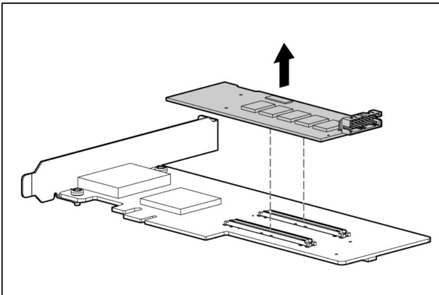
7. Install the new cache on the controller. Press firmly above each connector to ensure good electrical contact. (If the cache is not connected properly, the controller cannot boot.)
