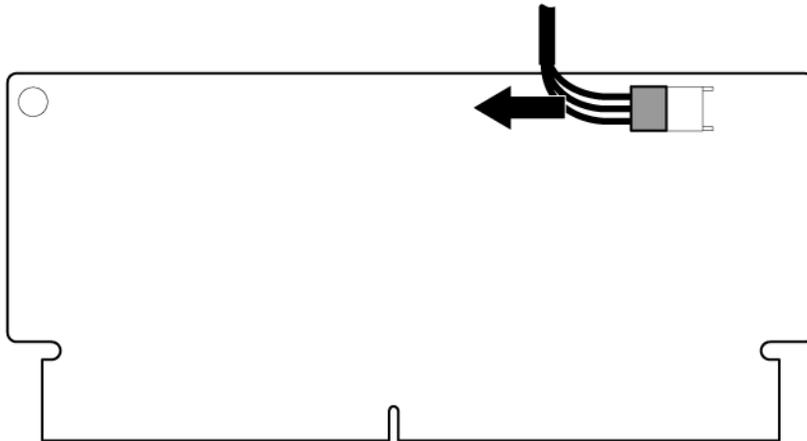
10. If the previous cache module was connected to a capacitor pack, **carefully** connect the capacitor pack cable to the new cache module.
