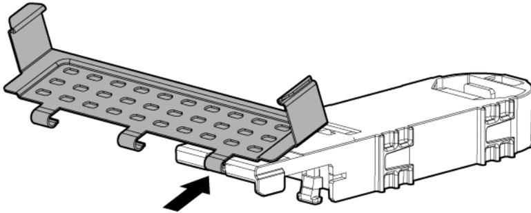
8. Align the posts on the bottom of the capacitor pack with the hole and groove on the controller.
