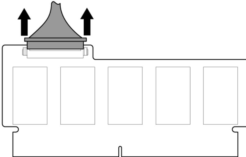
9. If the previous cache module was connected to a battery, connect the battery cable to the new cache module.
