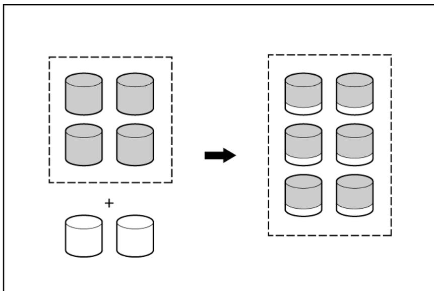
When the expansion process has finished, you can use the liberated storage capacity on the enlarged array to create new logical drives. Alternatively, you can use ACU to enlarge (extend) one of the original logical drives.
