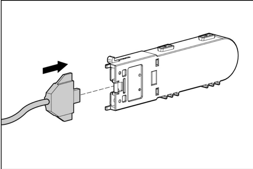
3. Install the new battery pack into the server. (The installation site depends on the server. For further information, refer to the server-specific user guide.)
