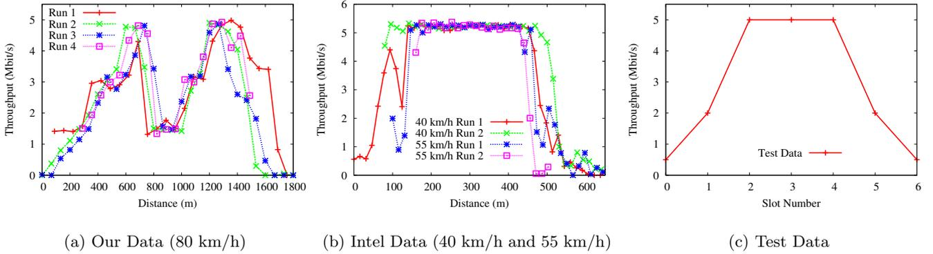
Figure 2: TCP Throughput over time (802.11b)
