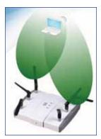
of phased array used in wireless access points: on-chip and onantenna, adopted by Cisco and Ruckus Wireless, respectively.
