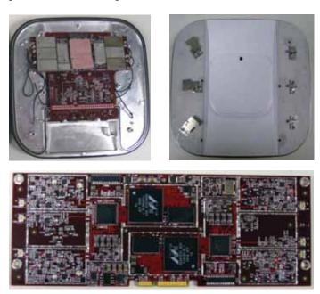
We also tested with an Aruba AP125 access point and Aruba 3200 controller with firmware 3.4.0.1 build 21611. There's not much to report here. This is a standard issue, enterprise-class, dual-band access point with three antennas you're never quite sure how to orient. The AP125 is pretty representative of "standard 802.11n,"
