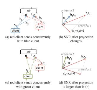
**Figure 1—Optimal bitrate changes after projection.** The optimal bitrate depends on the client that is transmitting concurrently. The smaller angle between the concurrent clients leads to a larger amount of SNR reduction after projection.
