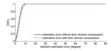
**Figure 9—Accuracy of direction estimation.** Leveraging channel reciprocity allows clients to measure the direction of the channels accurately in a passive way. The additional estimation error caused by compressing the time-domain channels is negligible.
