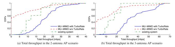
**Figure 11—Throughput Comparison.** The figure compares the throughput with and without TurboRate for the 2-antenna and 3-antenna AP scenarios. TurboRate delivers a total throughput gain of 1.7x and 2.3x as compared to existing 802.11. Without considering the effect of projection, the concurrent client in many cases selects a rate that makes its stream undecodable after projection and leads to zero throughput.
