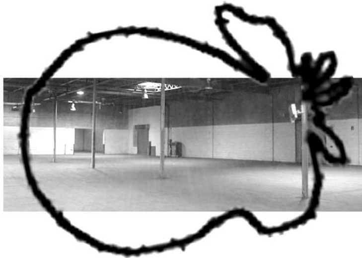
Figure 4.15 The Directional Antenna's Elevation Cut Seen in the Warehouse
