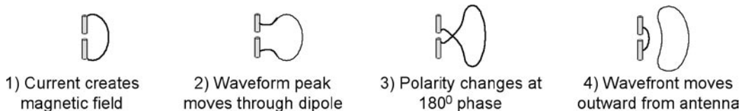
Figure 4.3 Wavefront Formation with a Dipole Radiator
