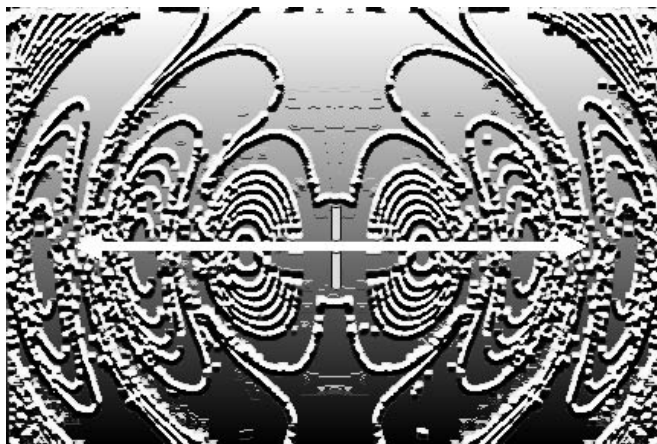
Figure 4.4 The Electromagnetic Field Surrounding a Dipole Antenna
