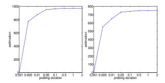
Fig. 3: Estimation of workloads generated by two traffic patterns following exponential distributions with mean of  $\frac{1}{973}$  and  $\frac{1}{751}$  respectively. X axis is different traffic measurement time from 0.001 seconds to 2 seconds. Y axis is the estimated workloads in packets per second.
