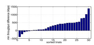
Fig. 8: Simulation result for 10 clients and 3 APs within  $30 \times 30$ . The simulation repeated 30 times. Each bar is the representative of minimum throughput difference for each trial. The results are sorted in ascending order
