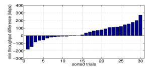
Fig. 10: Simulation result for 30 clients and 9 APs within  $150\times150$ . The simulation repeated 30 times. Each bar is the representative of minimum throughput difference for each trial. The results are sorted in ascending order
