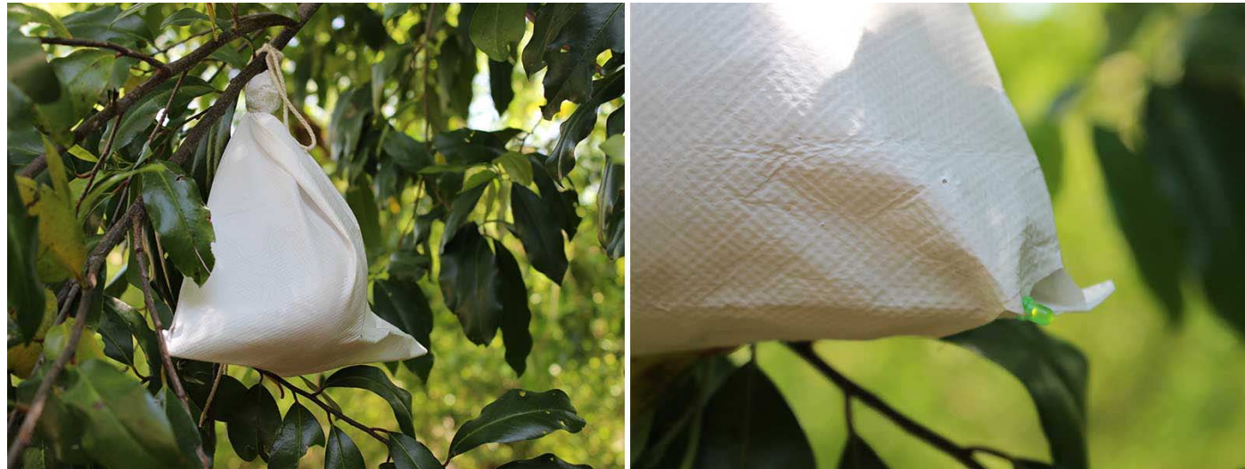
Figure 3 Ripeness detector. The detail at right shows the LED that lights up when the fruit is ripe.
