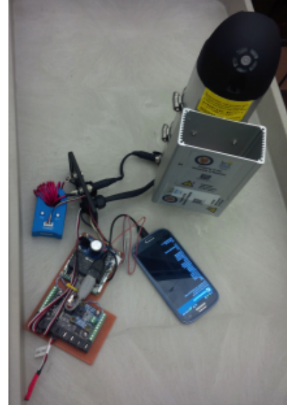
Figure 2: Sensor kit for the WeBike project
