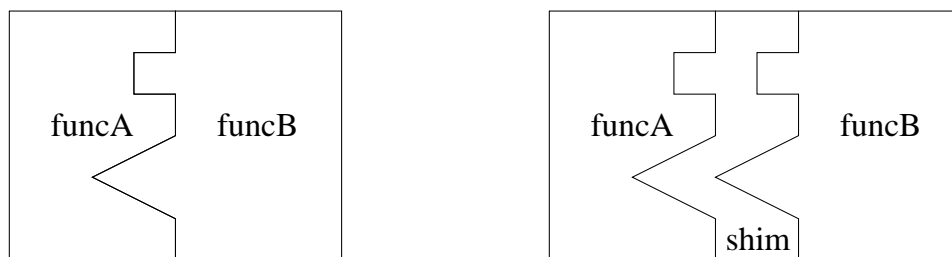
Figure 3: Using shims to insert instrumentation code (diagram from [41])
