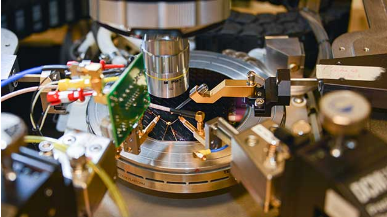
Photograph by Richard Lewington/Hewlett-PackardA memristor characterization experiment at HP Labs
