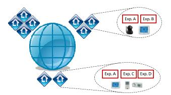
Figure 1: HomeLab would consist of multiple sites across the world. Each site has multiple homes and is deployed by a research group. Each home runs one or more experiments and contains one or more devices needed for the experiment.
