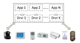
Figure 2: HomeOS is a platform that runs on a PC. Software modules called drivers communicate with devices and offer to applications high-level APIs to sense and actuate those devices.
