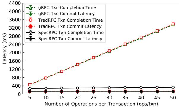
**Figure 9: Mean latency versus the number of operations per transaction with YCSB+T.**
