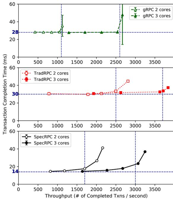
**Figure 13: Average transaction completion time versus throughput with Retwis.**
