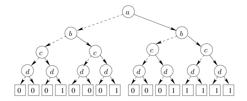
OBDT's are still exponential in the number of variables: Given n variables the OBDT's will have  $2^{n+1} - 1$  nodes! We can reduce the size of OBDT's by a recursive applications of the following reductions:
