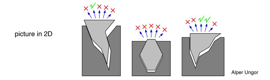
Pour liquid into a mold, harden, and then remove by straight line motion in some direction. Find a direction that works.
